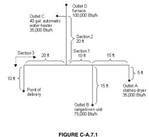
PIPING PLAN SHOWING A STEEL PIPING SYSTEM
