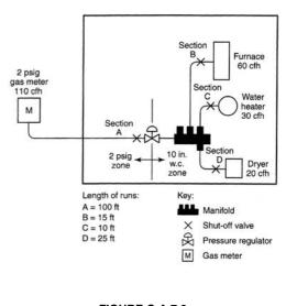
FIGURE C-A.7.2 PIPING PLAN SHOWING A CSST SYSTEM
