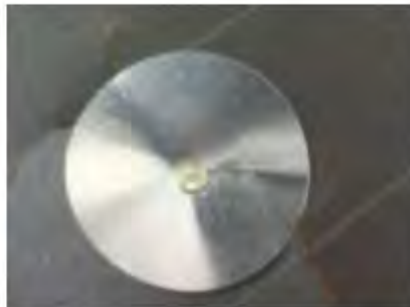
Metal cap with roofing nail fastener after the pull-through test. Observe the permanent deformation of the metal cap and the pull-through tears in the underlayment.
