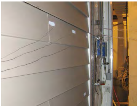
This is a photo of a test chamber and insulated siding being tested to ASTM C1363.
