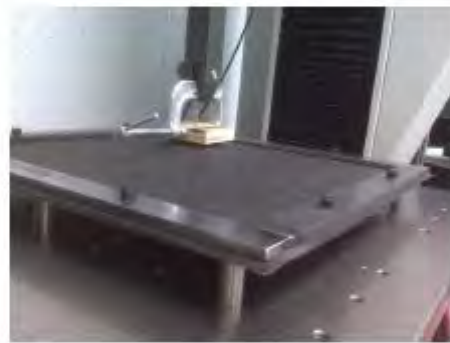
Pull-through test in progress; (left) early in test; (right) nearing failure.
